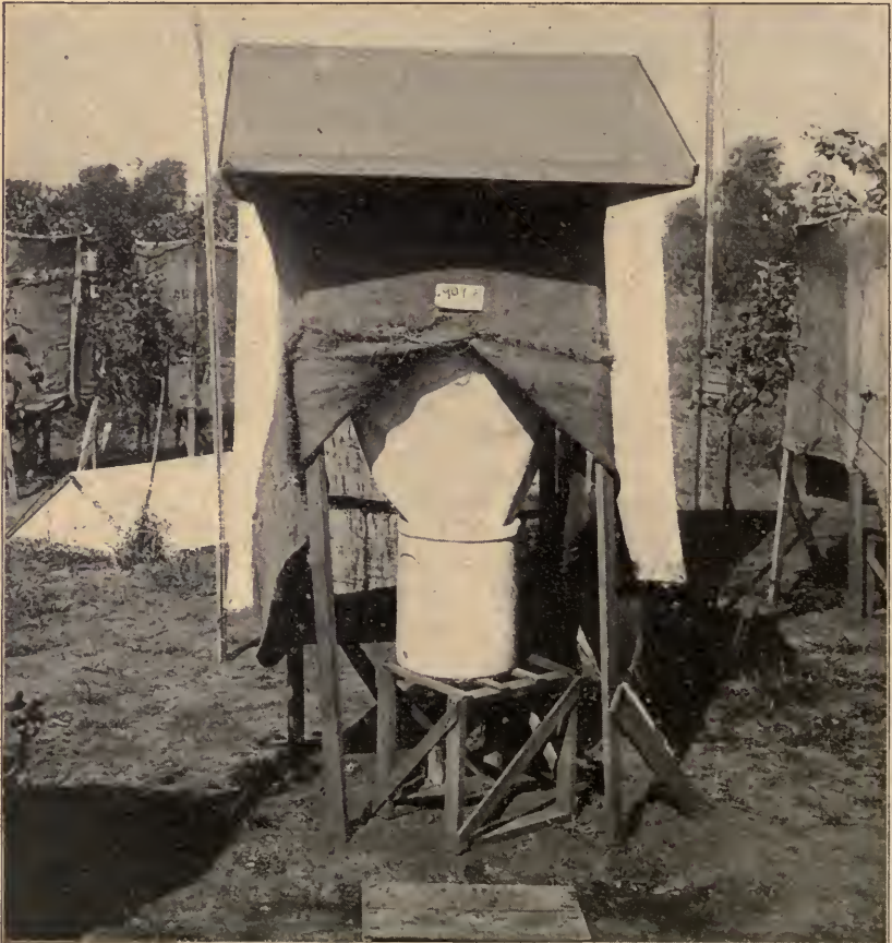
FIG. 8. Tree 907A, covered. Curtain raised to show drip jar. From photograph October 17, 1907.
